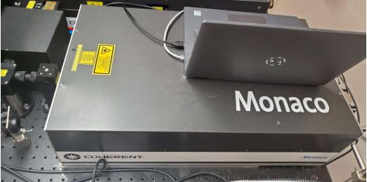
This Instrument is used as the two laser sources for the SEE Instrument. Supports single and double photon excitation
