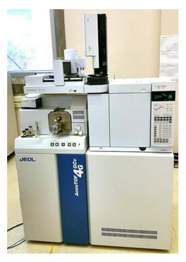
The JEOL mass spectrometer is a High-Performance Gas Chromatograph Time-of-Flight Mass Spectrometer. It is interfaced with an Agilent 7890A Gas Chromatograph with auto sampler. It is equipped with an EI only source and an EI/FI combination source that is capable of field desorption. GCMS in EI mode a NIST library can be used to help identify chromatography peaks.
