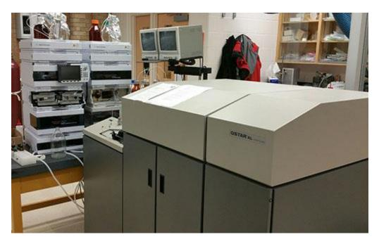
QSTAR XI LC/MS/MS mass spectrometer is a quadrupole / Time-of-Flight mass spectrometer with an ESI source. This high-resolution MS/MS has the capability for exact mass measurement. Samples are introduced into the mass spectrometer either by infusion or using an Agilent 1100 LC system. Also available is an Agilent 1260 Nano LC system that the samples can be analyzed with a Nanospray source.
